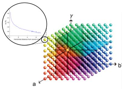
Figure 1. Conceptual representation of a look up table. Every points represent a simulated reflectance curve for a given set of IOPs ( $a$ ,  $b'$  and  $\gamma$ ).
