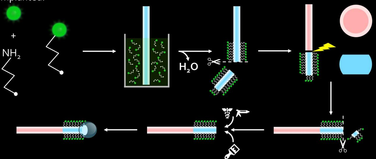
Figure 5. FITC functionalized with APS is used to graft fluorophores to the fiber surface. It is then cleaved, spliced with a multimodal 105/125 fiber, cleaved to appropriate length and capped with medical silicone and paint.
